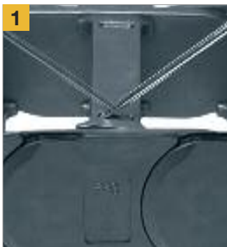
1 Remove crossbars - Insert screwdriver into the slot, using a lever action, apply pressure to the screwdriver to remove the crossbar.
