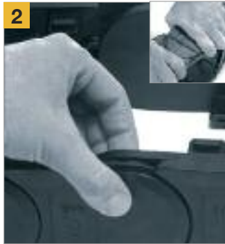
2 Join the side links - join the second side link by pressing from the top
