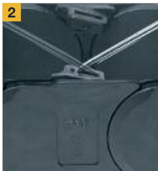
2 Remove clips - Insert screwdriver into the slot, using a lever action, apply pressure to the screwdriver to remove the clip
